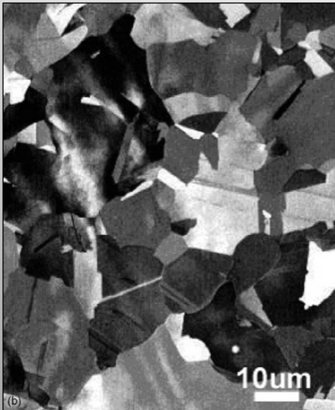
Recrystallized grains observed in HE plate-impacted Cu (001) and (221) at 57 GPa but not observed in laser shocked samples
